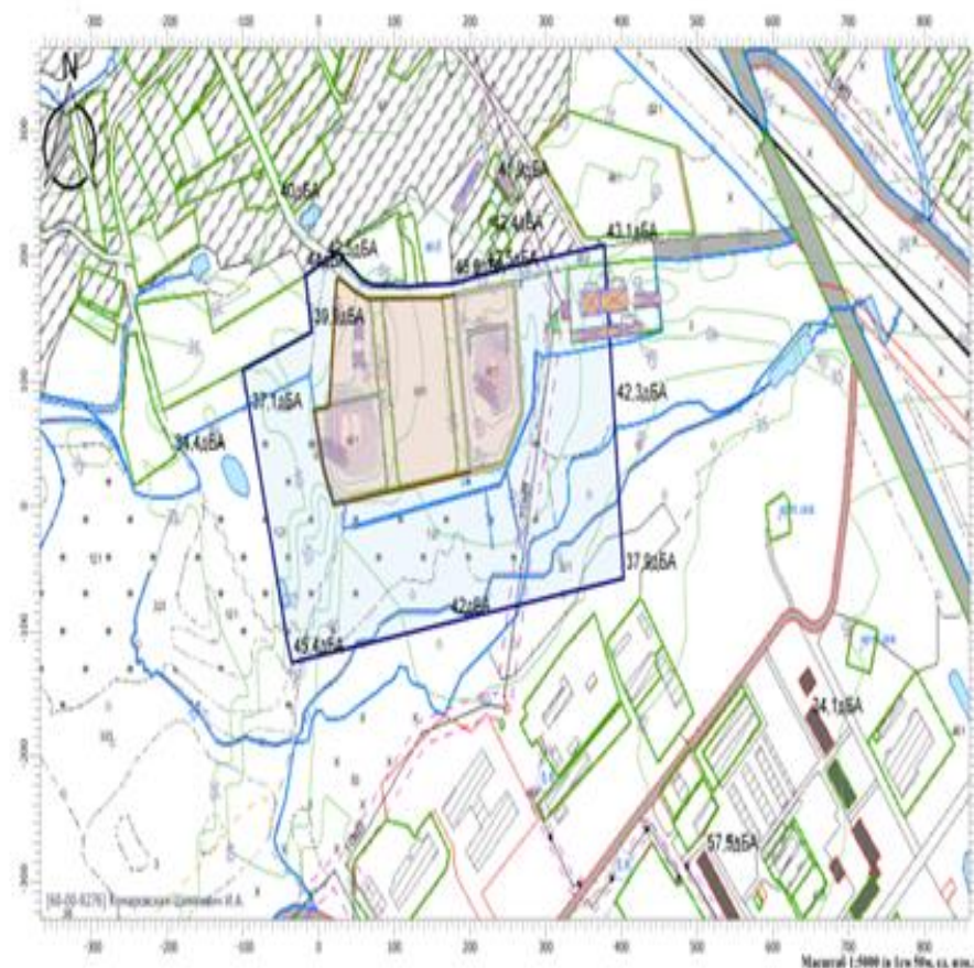
Evaluation of the equivalent sound level (dBA) at the border of the sanitary protection zone and beyond
